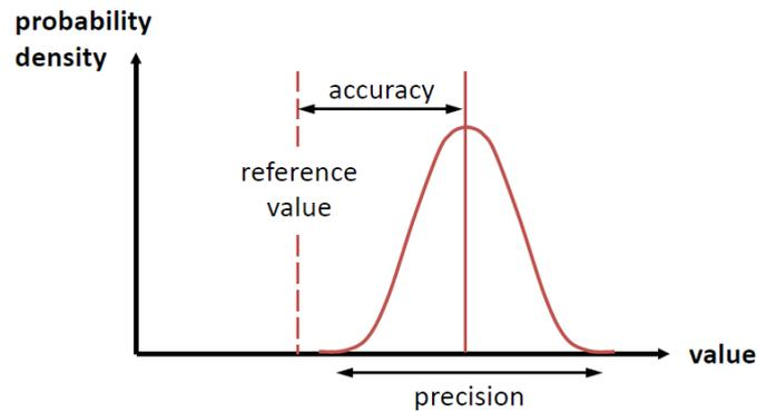
Figure M-1: Illustration of precision and accuracy in measurement (source: DLR).
