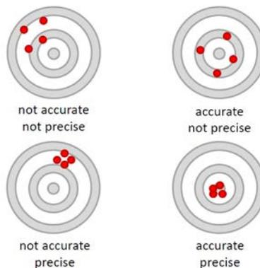
Figure M-2: Illustration of independence of accuracy and precision for an exemplary measurement. (source: DLR)
