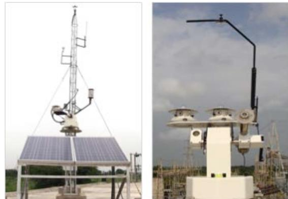
**Figure 2:** Typical SRRA station design (left); solar tracker with pyrhemeter and platform to carry pyranometers and shading assembly (right).
