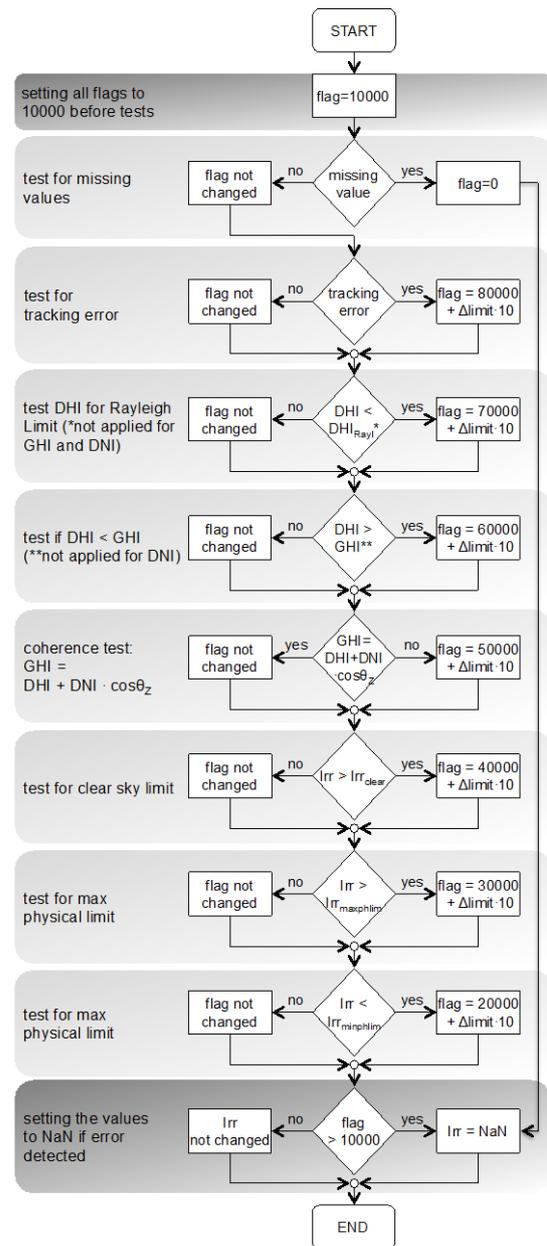
**Figure 4:** Flow chart showing the various tests performed on three major solar radiation parameters GHI, DNI and DHI.
