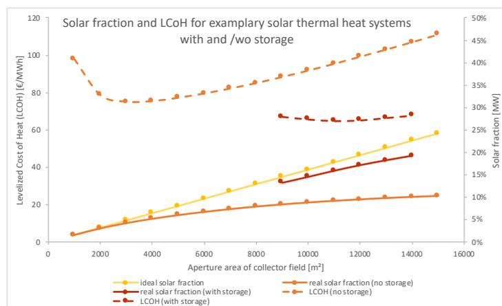
The first application was a general examination of the techno-economic feasibility of solar thermal plants in Germany. The influences of different locations, different heat grid temperature levels and varying system configurations were examined. It could be shown that even small buffer storages are able to increase the yield of the collector field by at least 80% compared to systems
