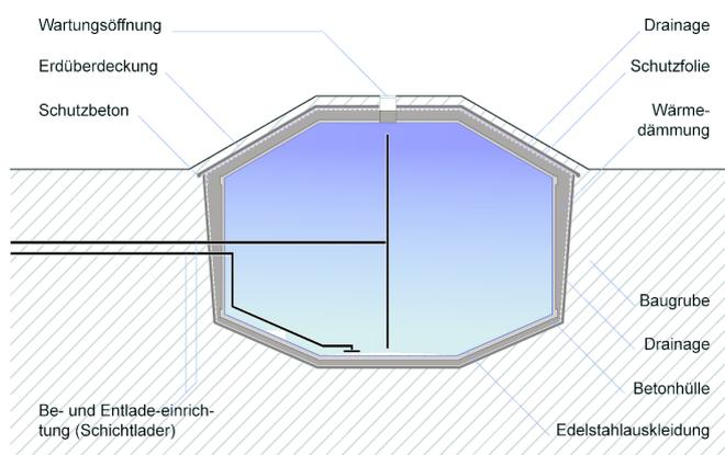
Figure 1 - Typical pit thermal energy storage
