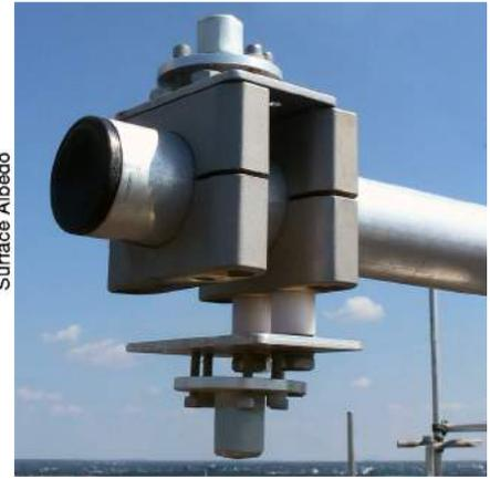
Albedometer with two photodiode pyranometers
