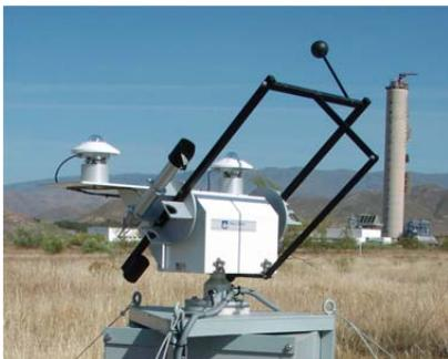
Figure 2: Meteorological station with highly precise instrumentation: 2 pyranometers (GHI, DHI), pyrliometer (DNI) and shadow ball, mounted on a 2AP solar tracker.
