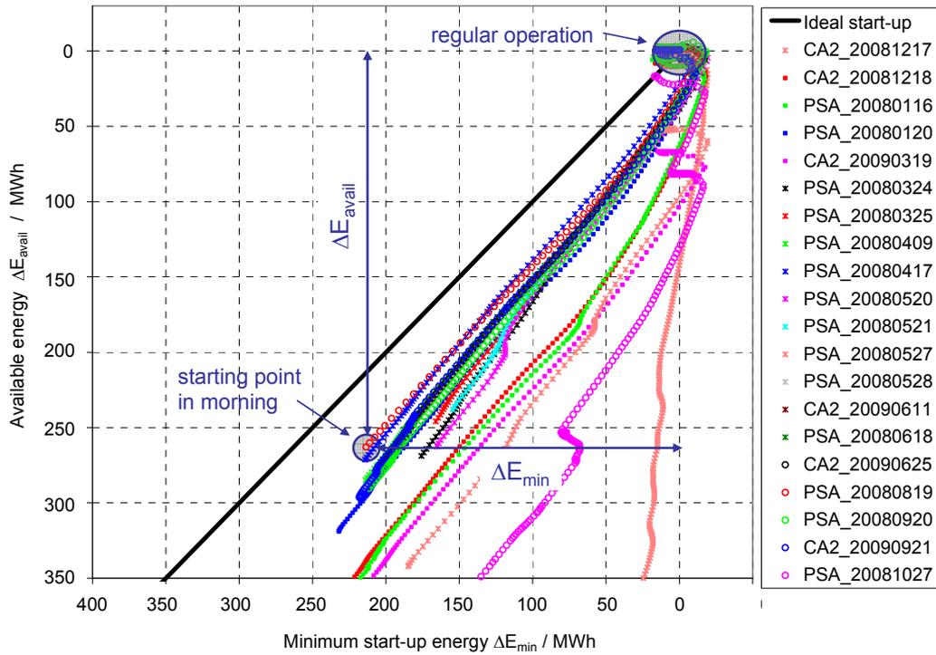
Fig. 1. Start-up diagram for various days obtained from dynamic simulation
