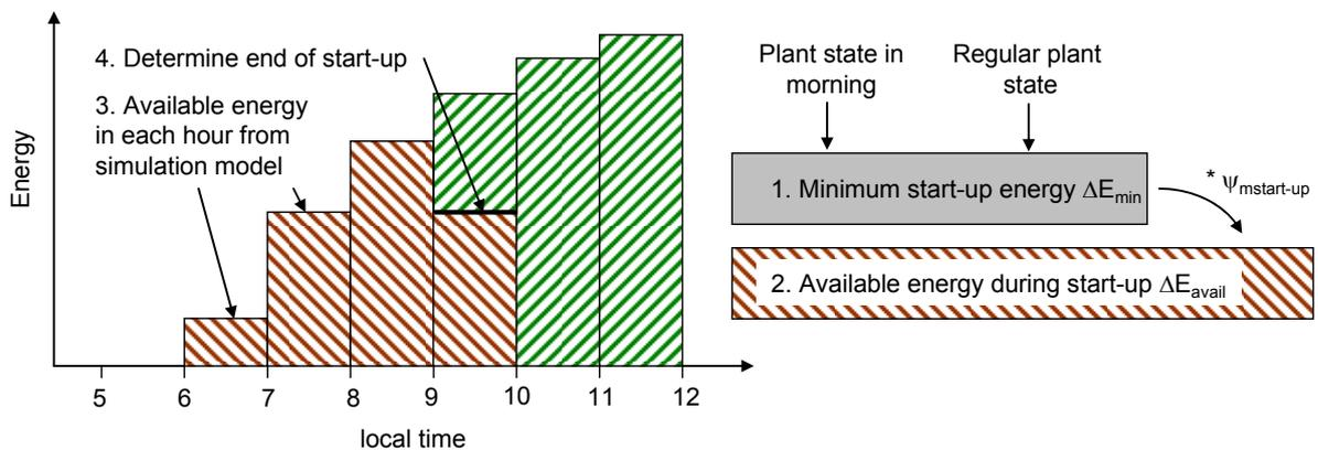
**Fig. 3. Approach to consider start-ups in steady-state simulation models**
