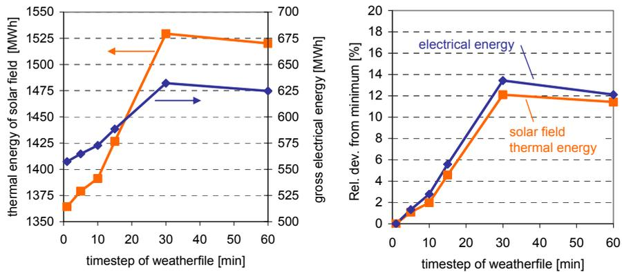
Fig. 5. Impact of weather data resolution on daily energy yields on April 11<sup>th</sup>, 2008
