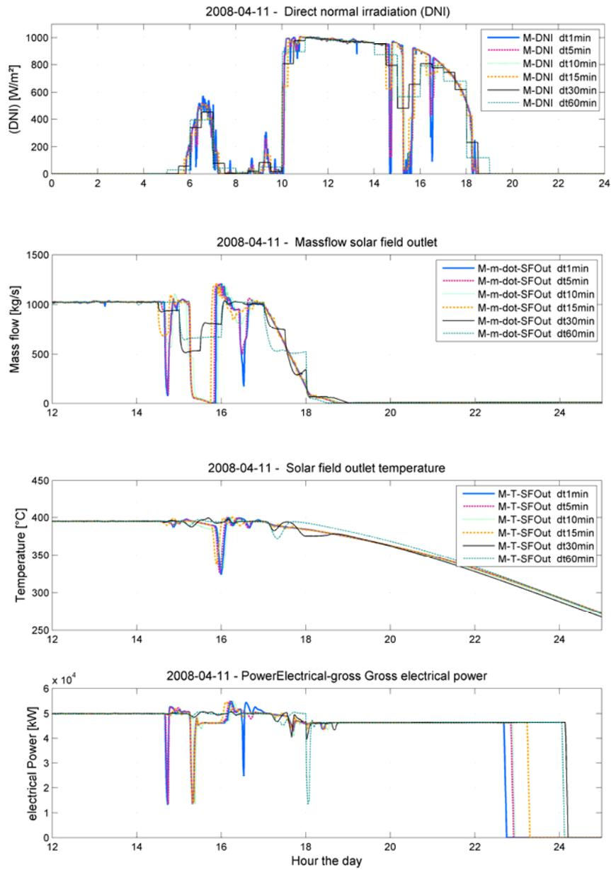
Fig. 4. Simulation results for April, 11<sup>th</sup>, 2008 on PSA for different temporal resolutions
